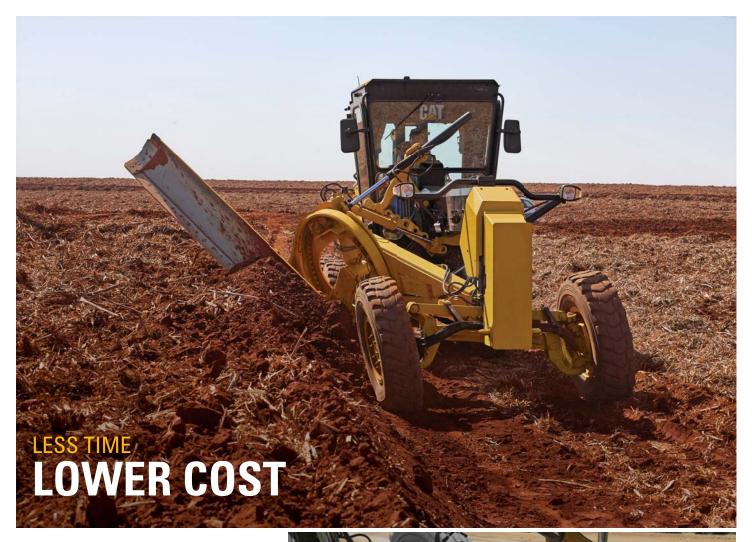
Keep your circle moldboard tight for precise grading throughout the motor grader's life. Durable structures with drawbar circle moldboard adjustments save you service time using replaceable wear inserts.
